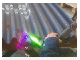
3D SCANNING FOR REVERSE ENGINEERING (HEXAGON ARM & 3D LASER SCANNER)
